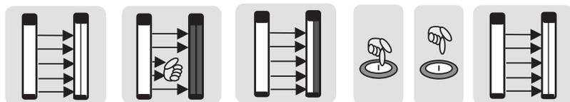
**Fig. 4.2-2:** Start/restart interlock function after interrupting the protected field
