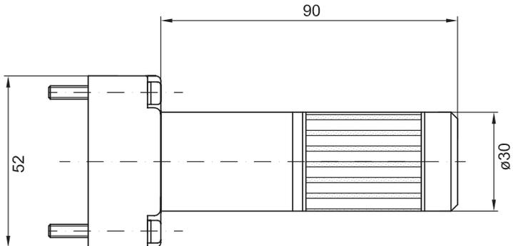
**Fig. 12.2-6:** Option: Integrated LED muting lamp
