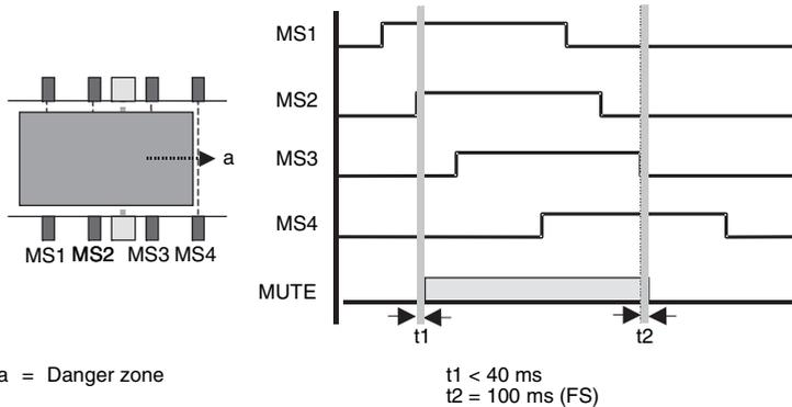
**Fig. 4.3-1:** 4-Sensor Sequential Muting
