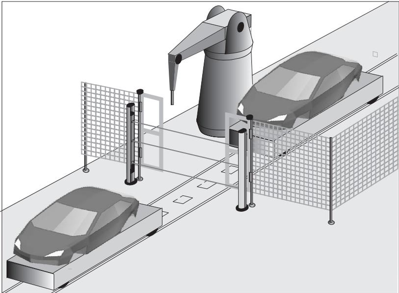
Fig. 3.4-1: Multiple Light Beam Protective Device, muting application at a robot station
