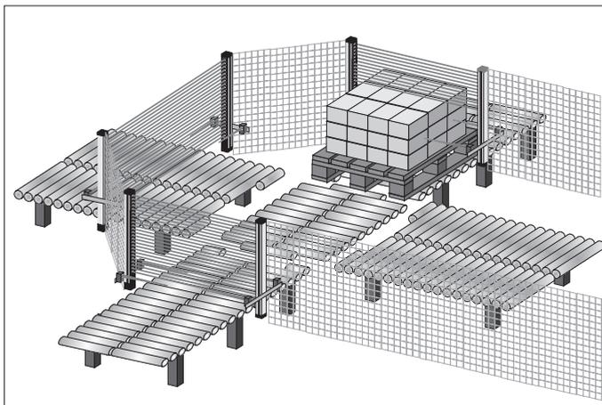
**Fig. 3.4-3:** Safety Light Curtain, muting application on a conveyor system
