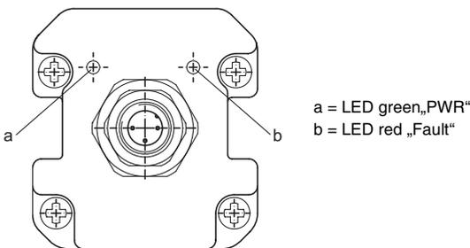
**Fig. 7.9-4:** Receiver/Transceiver connection cap with LEDs
