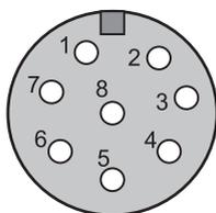
**Fig. 7.1-1:** Receiver/transceiver – local connection socket M12, 8-pin
