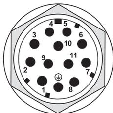
**Fig. 7.7-1:** Receiver/transceiver machine interface /R2, Hirschmann plug (view of the pins)
