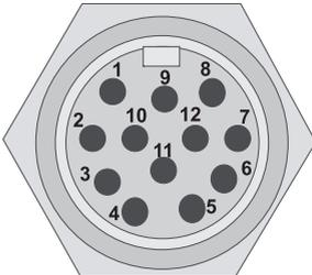
**Fig. 7.8-1:** Receiver/transceiver machine interface /R3, MIN-series (view of the pins)
