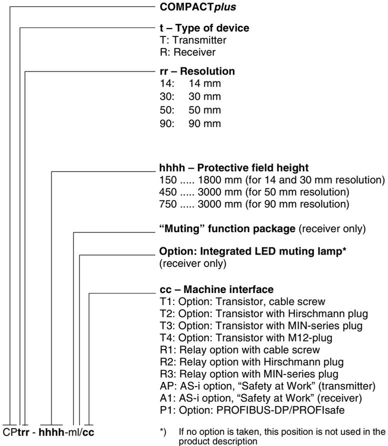
**Fig. 1.3-1:** Selecting COMPACTplus-m Safety Light Curtains
