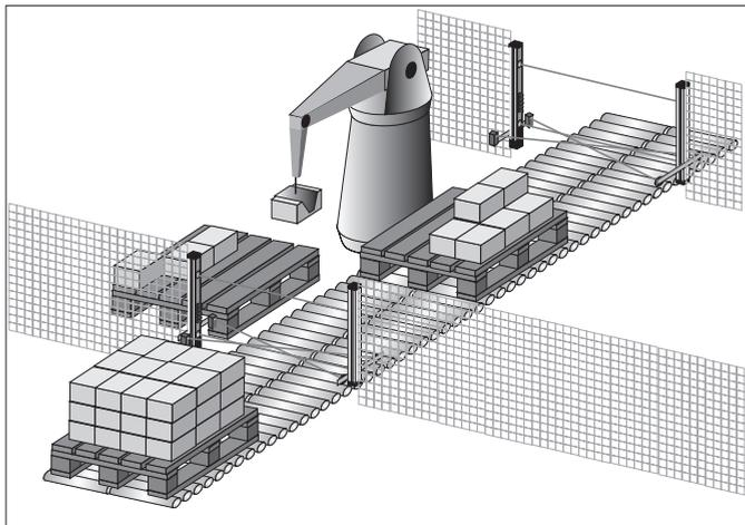
**Fig. 3.4-2:** Muting Transceiver, application on a palletizer
