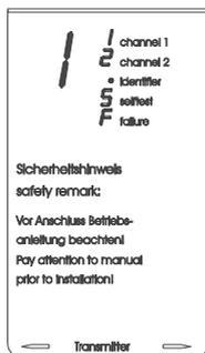
Fig. 5.1-1: Transmitter status displays
