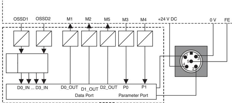
**Fig. 7.9-5:** Machine interface /A1, schematic structure
