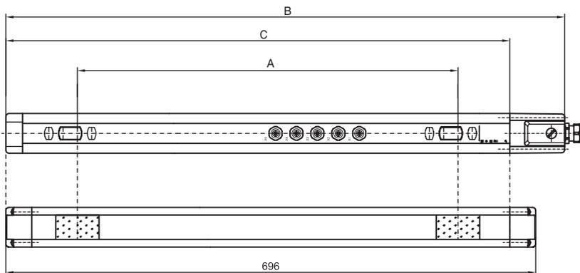
**Fig. 12.2-3:** Muting transceiver dimensions
