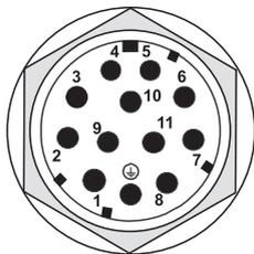
**Fig. 7.3-1:** Transmitter and receiver/transceiver, machine interface /T1 (view of the pins)
