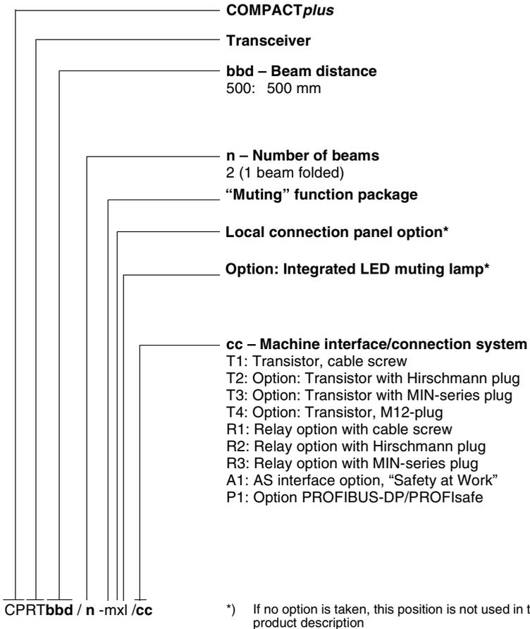
**Fig. 1.3-3:** Selecting COMPACTplus-m Muting Transceiver
