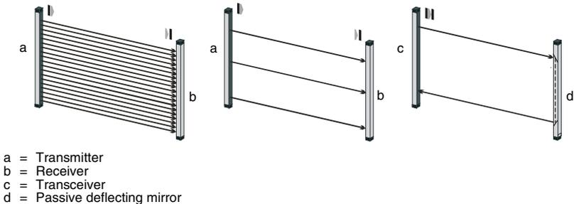
**Fig. 3.1-1:** Principle of the opto-electronic protective device
