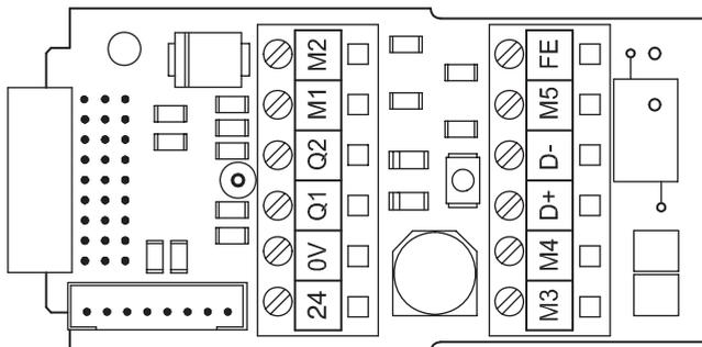
**Fig. 7.2-3:** Receiver/transceiver machine interface /T1, terminal field
