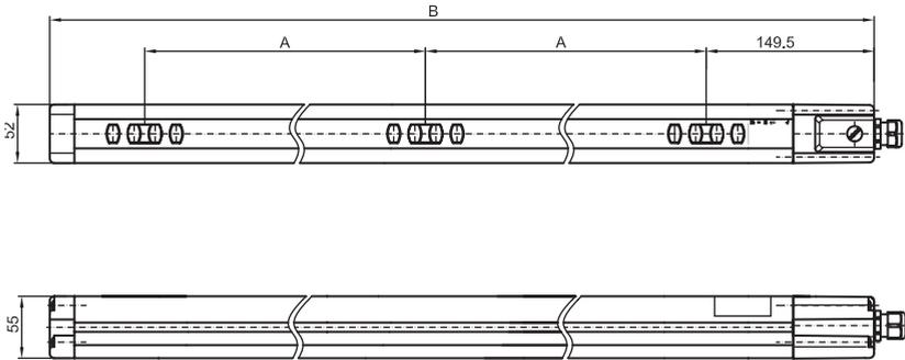
**Fig. 12.2-2:** Multiple light beam protective device dimensions
