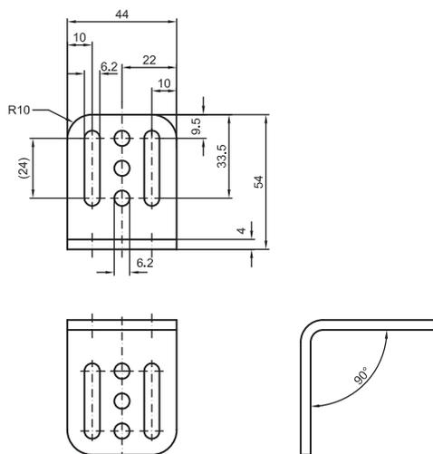
**Fig. 12.2-4:** Standard mounting bracket
