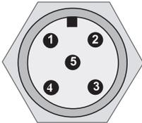
**Fig. 7.9-3:** Receiver/transceiver machine interface /A1, 5-pin M12 plug signal assignment
