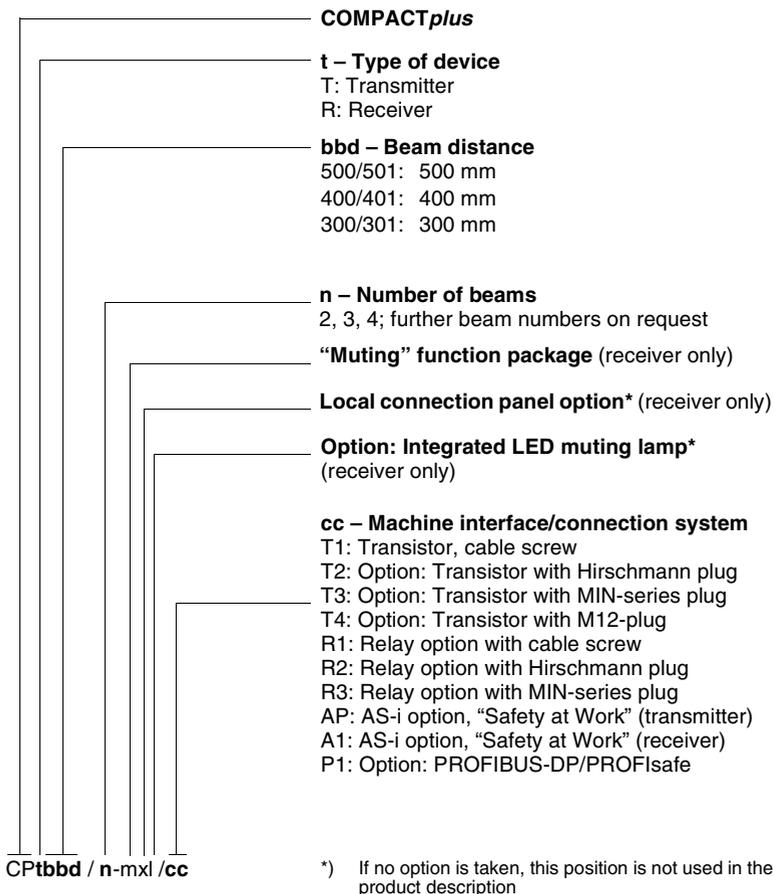
**Fig. 1.3-2:** Selecting COMPACTplus-m Multiple Light Beam Protective Devices
