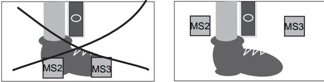
**Fig. 6.1-4:** Arrangement of the muting sensors MS2 and MS3
