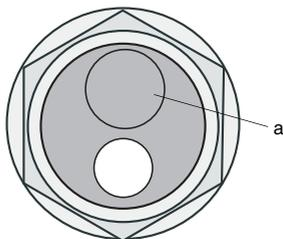
a = Just push opening through when a separate connection cable for the load circuit is to be connected.
